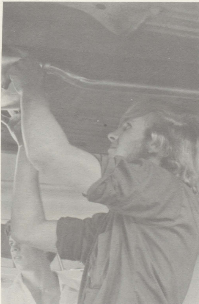
Curt Smith installs a new muffler in Mr. Santivicca's auto shop,
