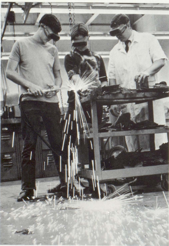
Mr. LaMagna looks on as Chris Merenuk and Dave Carey cut a piece of metal with an acetylene torch.
