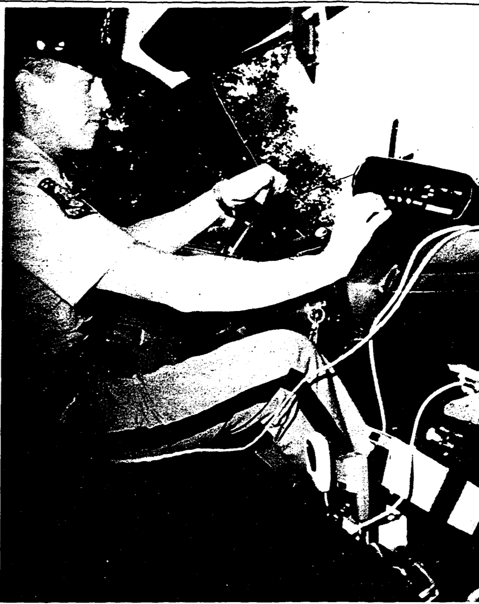
SPEED CHECK—Northville City Patrolman Bruce Deacon checks the speed of traffic with the city's radar unit. Purchased with funds received through a federal traffic safety grant, the radar unit has a range of 2,500 feet and speeds of vehicles can be "locked in" and recalled through the system's memory bank. Deacon is a member of the city's new traffic division headed by Sergeant Louis Westfall.
