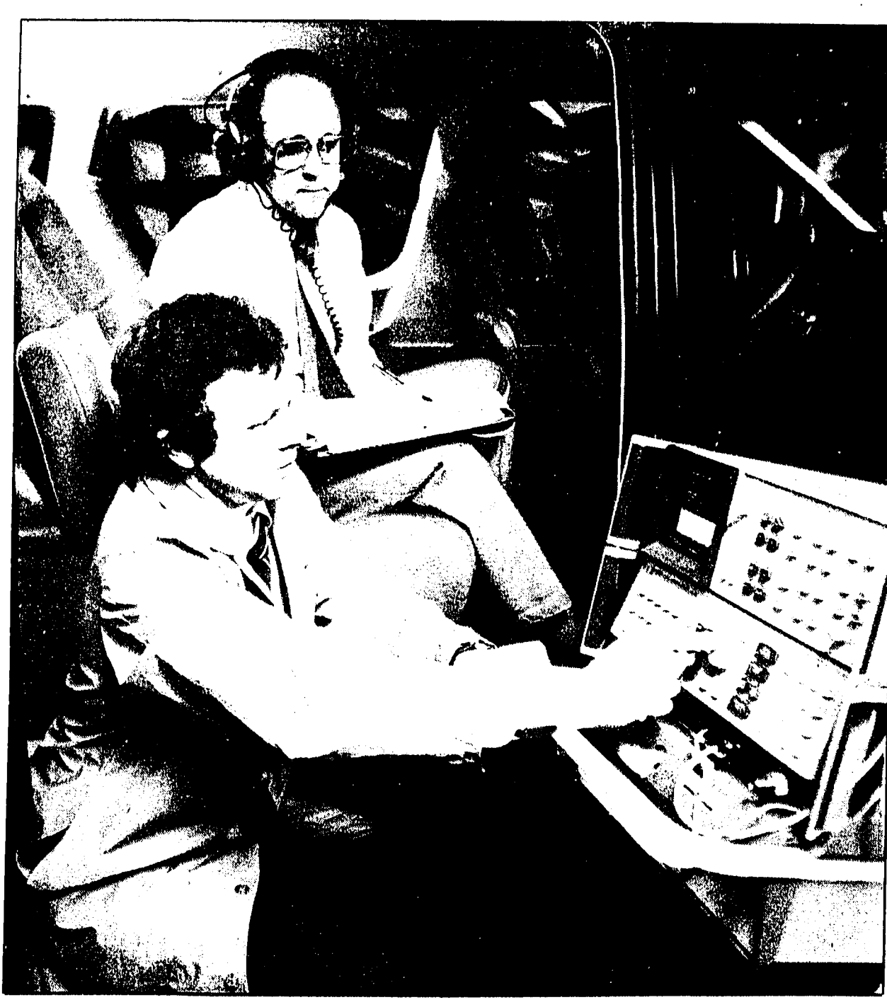
Ford audio-design engineers William C. Adamson (front) and William A. Forbes check for noise sources that might cause interference with radio reception on the Ford Aerostar's new "SuperSound" system in an anechoic chamber at Ford's Diversified Products Technical Center in Dearborn.
