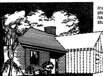
Includes: 2X8 floor joists, shingles, two sliding windows, nails, rustic fir siding and 3/4 T&G sturdy subfloor.
