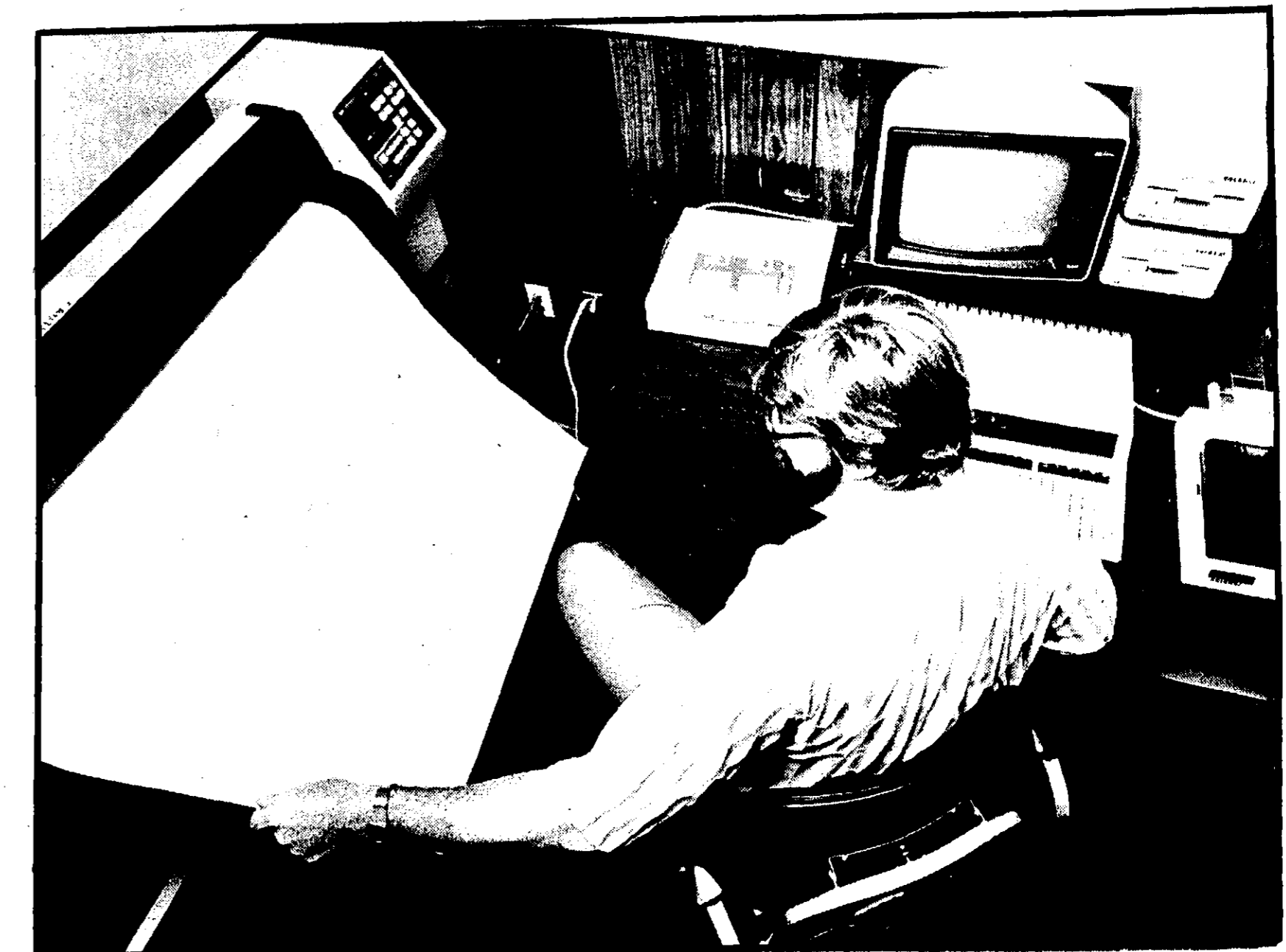
PLOTTING BY COMPUTER--A printing device called a plotter yield drawings of plans and specifications for road improvements which were developed with the help of a computer for Civil Engineer Charles Werner. Computer technology is being used increasingly to speed engineering functions.
