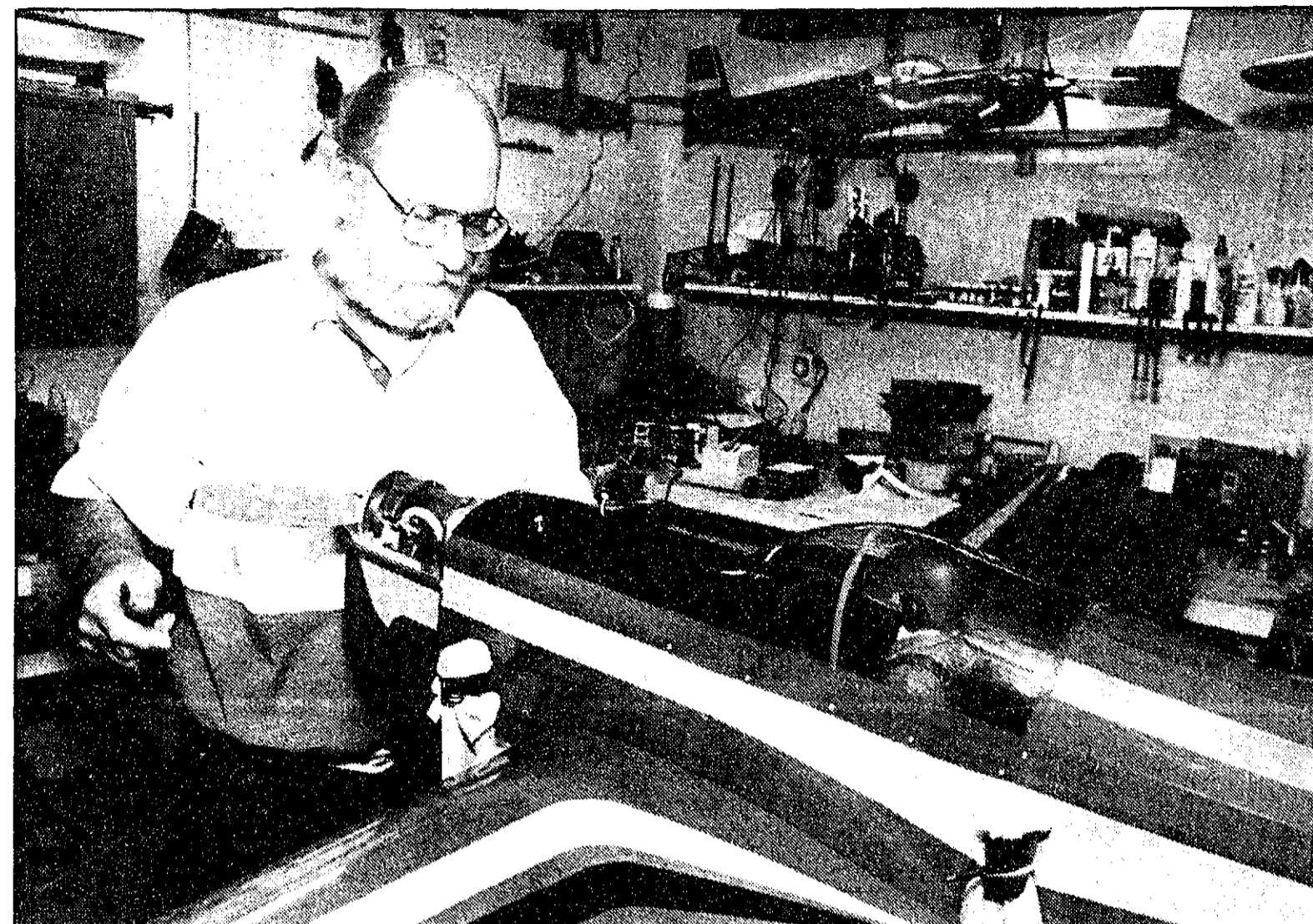
Dave Doehler, in his workshop in his Northville home, works on his "Pride and Joy." He calls this plane a cad-spot. He designed the plans on a computer, made a pattern and built it himself. It has a four horsepower chainsaw engine in it. He hopes to fly it soon.
