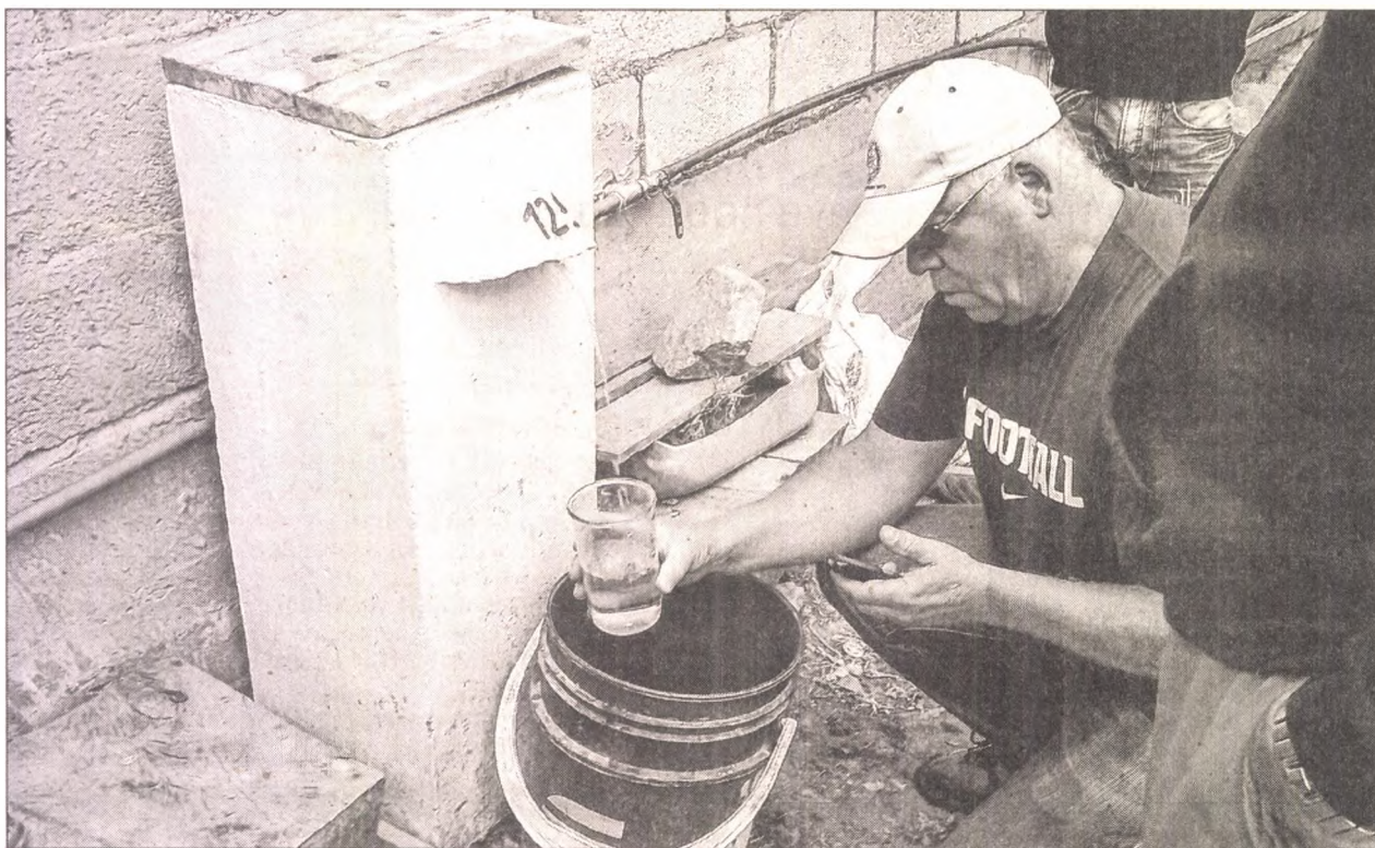
Gary Sobotta checking the flow rate of a filter to ensure proper pause time.
