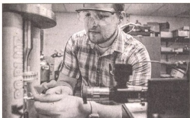
University of Michigan student Jake Adams re-attaches string gauges in an ultrasonic fatigue apparatus in the Gerstacker Building.
