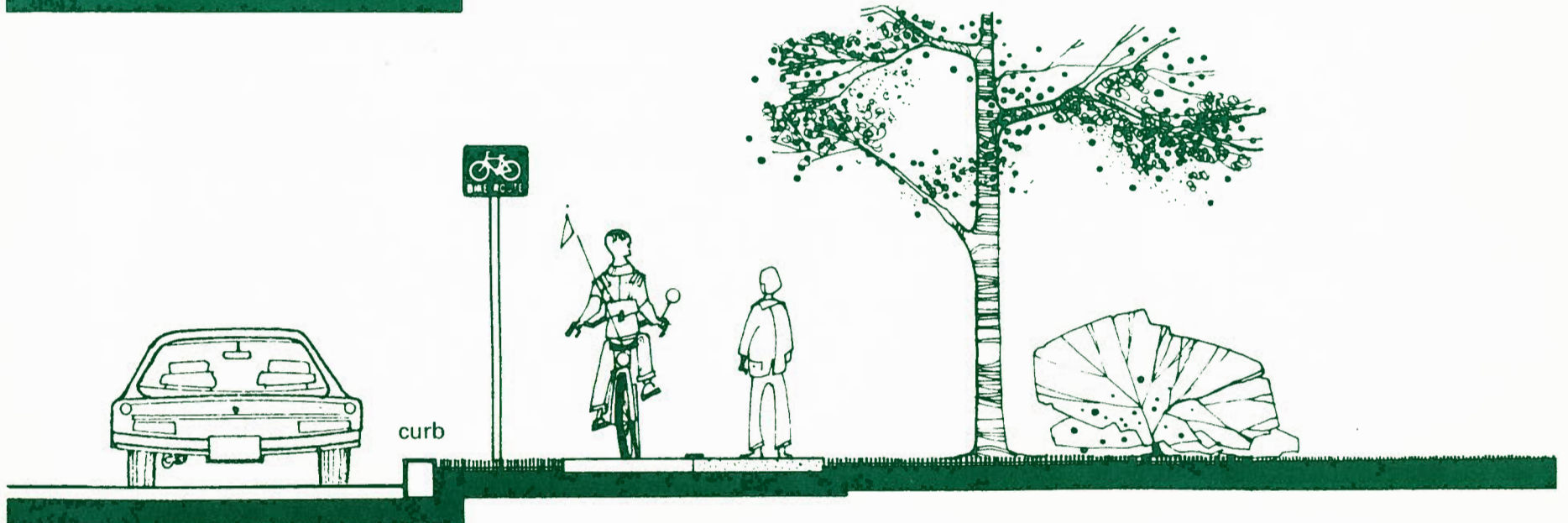
CLASS 1 - SHARED PEDESTRIAN/BIKE PATH SURFACE; WIDE PAVEMENT 10 FT. - 12 FT., WITH PAINTED DIVIDER OR CHANGE IN SURFACE MATERIAL.
