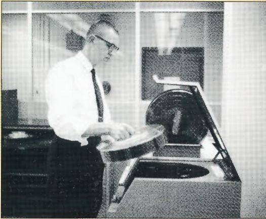
Senior Programmer, Dave McBroom installing magnetic storage disc.
