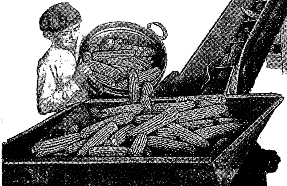
One of the small grain elevators can store five hundred bushels of ear corn an hour—for a penny's worth of electricity!
