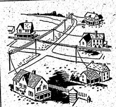
HARD-WORKING WIRES - Helping to bring telephone service to more farm families is the application of "carrier" equipment to rural telephone lines. This special equipment, used for years on Long Distance lines, enables several conversations to travel along the same pair of wires at the same time and without interfering with each other. Recent developments indicate that, under suitable conditions, extra rural circuits also can be provided in this manner.
