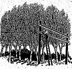
BARK THAT BITES - To test various types of insulating coatings for telephone wires, Bell Laboratories maintain a dense birch forest in New Jersey. Wires strung through the forest show how different materials resist the rubbing action of tree limbs under actual outdoor conditions.
