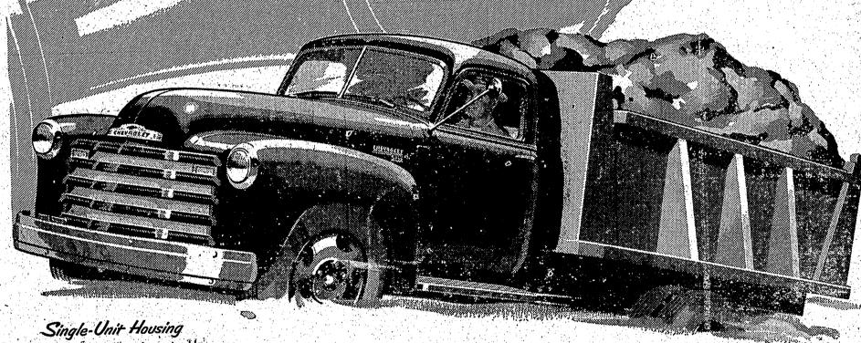
Here's maximum strength ... longer trouble-free service! Chevrolet rear axle housings are formed into tubular steel beams; no bolts or rivets to work loose.
