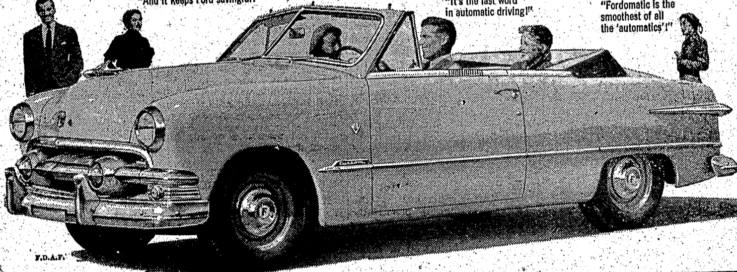
EASY "ROCKING" . . . even easier than with conventional drive. Just flip the selector back and forth between "Reverse" and "Low" . . . you'll find you're un-stuck from mud, sand or snow in 1/2 minute.
