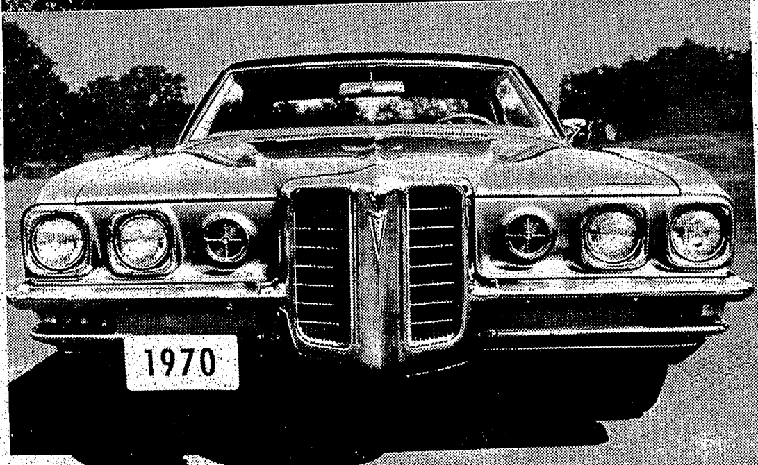
Front end styling of the big Pontiacs reflects the influence of the pace-setting Grand Prix (top) and its classic vertical center grille as shown on this 1970 Bonneville. The horn grilles between the center grille and headlamps not only serve as outlets for the sound of the horns, but also admit additional engine cooling air. The Bonneville is powered by a new 455 cubic-inch engine that also is offered as an option on the Grand Prix. All 1970 Pontiacs go on sale September 18 at Jack W. Haupt Pontiac Sales and Service, Clarkston.
