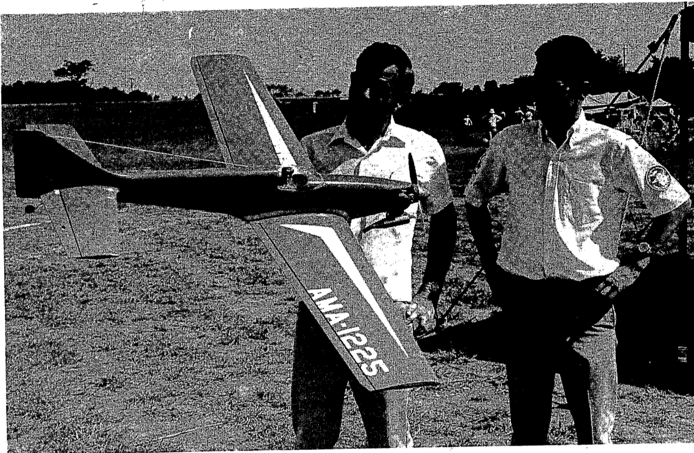
It'll do 110—Radio controlled model planes competed in Clarkston this weekend. They came from all over the U.S., east of the Mississippi. Paul A. Schmitz of Monroe holds his for the camera. It weighs 7½ lbs., burns alcohol, nitromethane and castor oil, has 1½-hp, turns 12,000 rpm's, and will do 110 mph. and has a retractable landing gear. Roy Pinner, of Waterford, and president of the contest sponsoring Pontiac Model Airplane Club, is with Schmitz.
