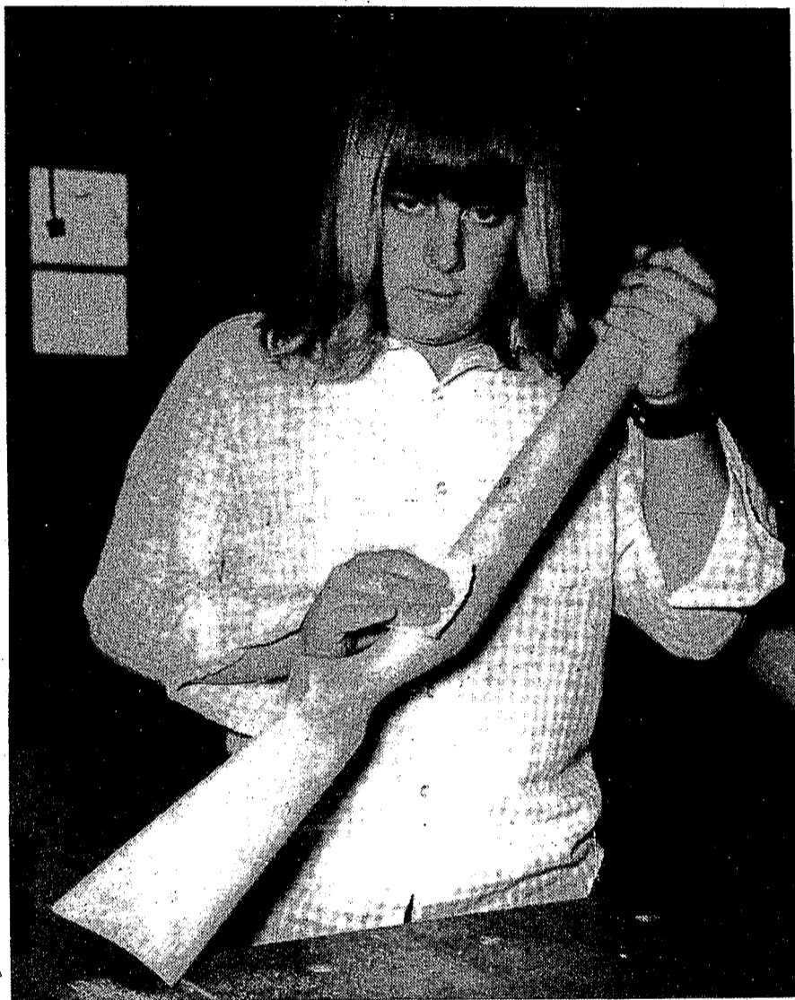
Ron Tunningley refinishes the stock of his 22 rifle in woodworking classes at Sashabaw Junior High. He's removed the old finish, is now sanding, and about ready to apply a new walnut stain.
