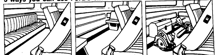
Foam-padded rear seat (optional) folds flat like a station wagon's to make load floor for cargo. Facing jump seats (optional) have foam-padded cushions and backs, fold out of way for cargo. Big 44-cu. ft. cargo space is easy to reach from either side of split-back front seat with low flat floor.
