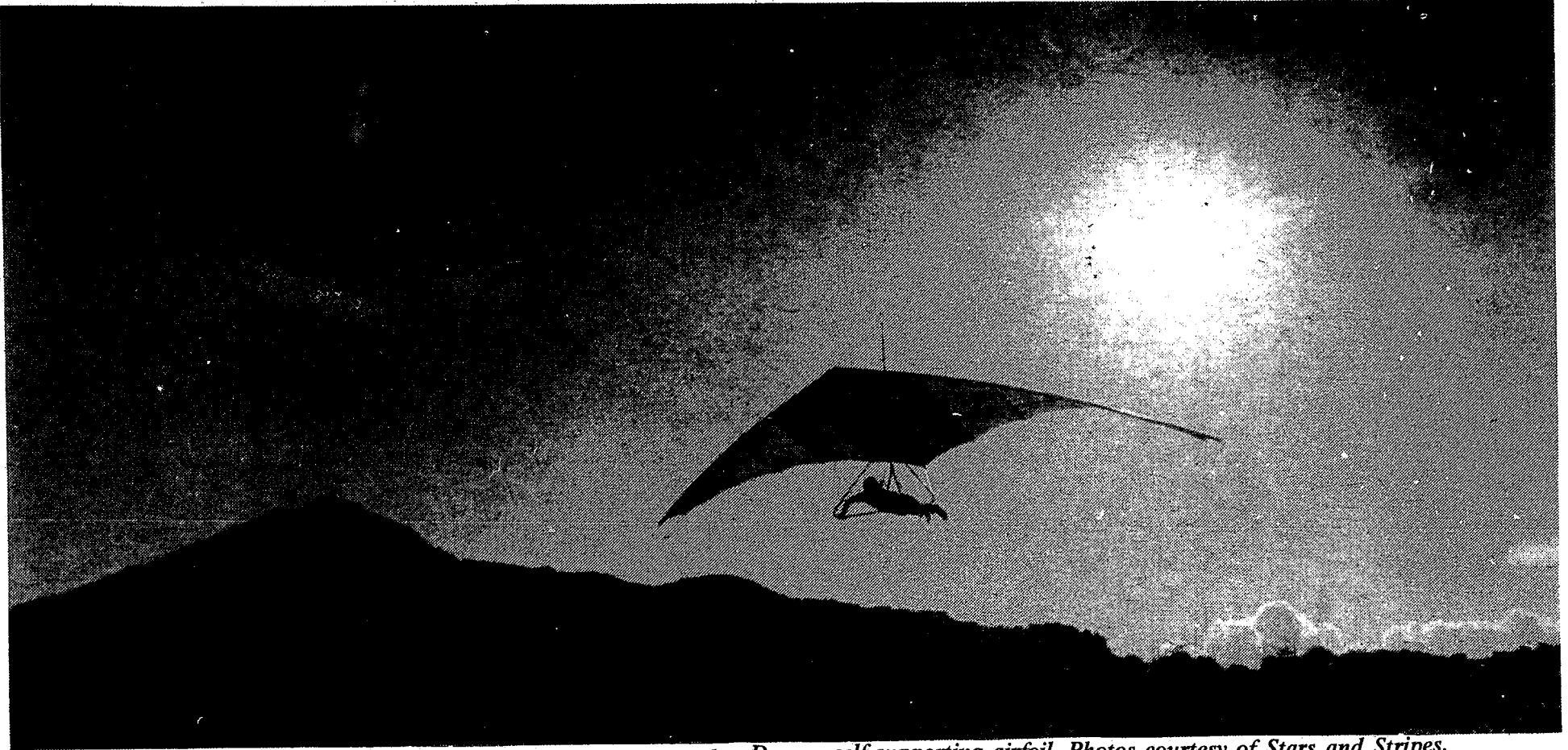
Rick Leaf sails through the air under his aluminum-and-Dacron self-supporting airfoil. Photos courtesy of Stars and Stripes.
