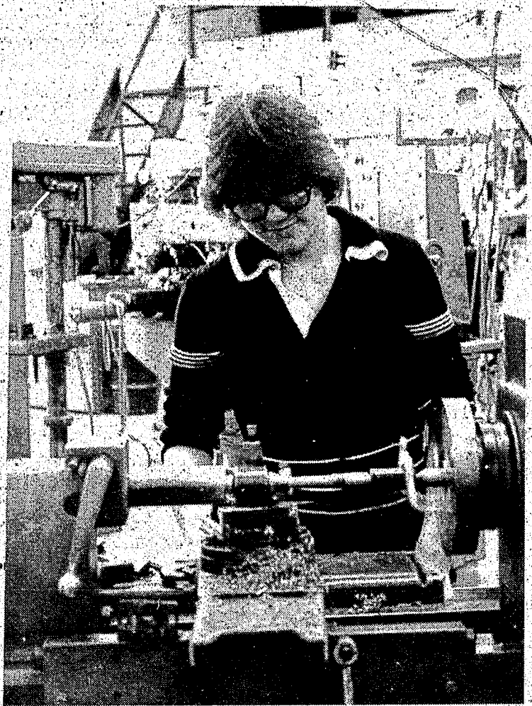
Grinding a spring-loaded center for a tail stud is part of Clarkston High student's Ray Chevalier daily training in the Northwest Vocational Education Center's machine shop classes.
