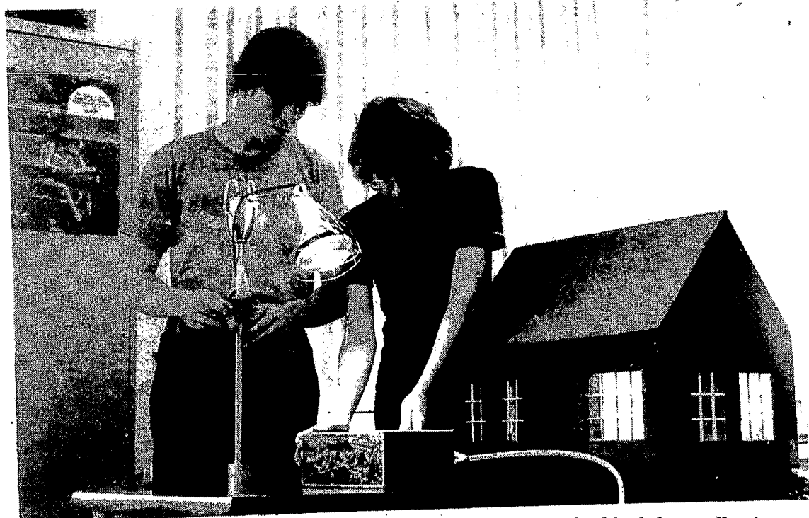
As Scott Temple peers over a sunlamp, Scott Smith adjusts the black box collecting heat to warm the boys' blue-ribbon winning solar house.
