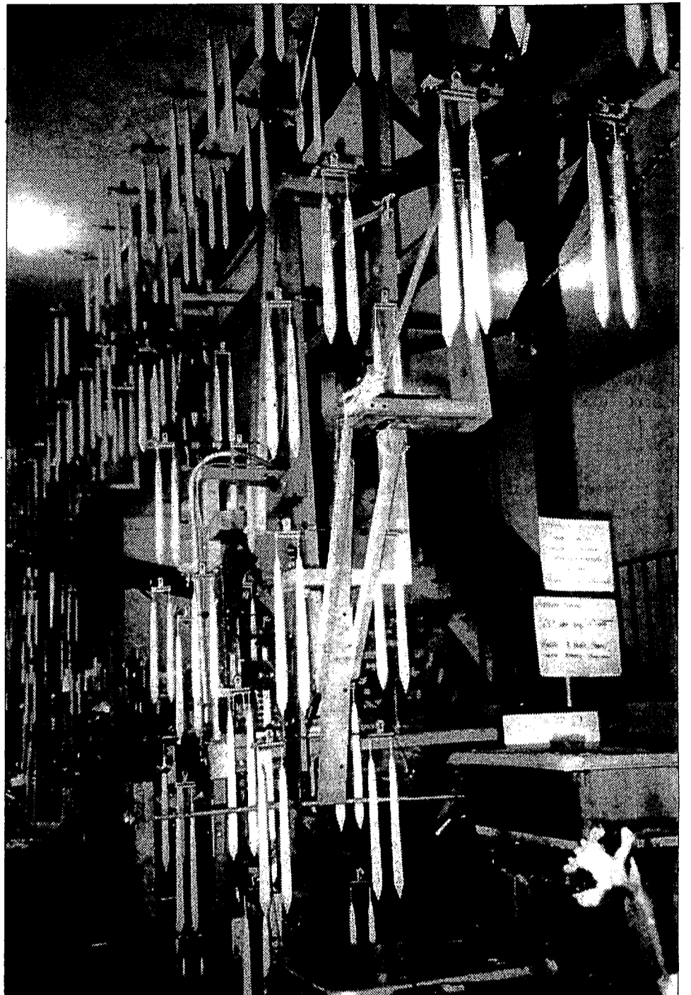
The taper line stocked with candles after dipping them repeatedly for over three hours. Photo provided
