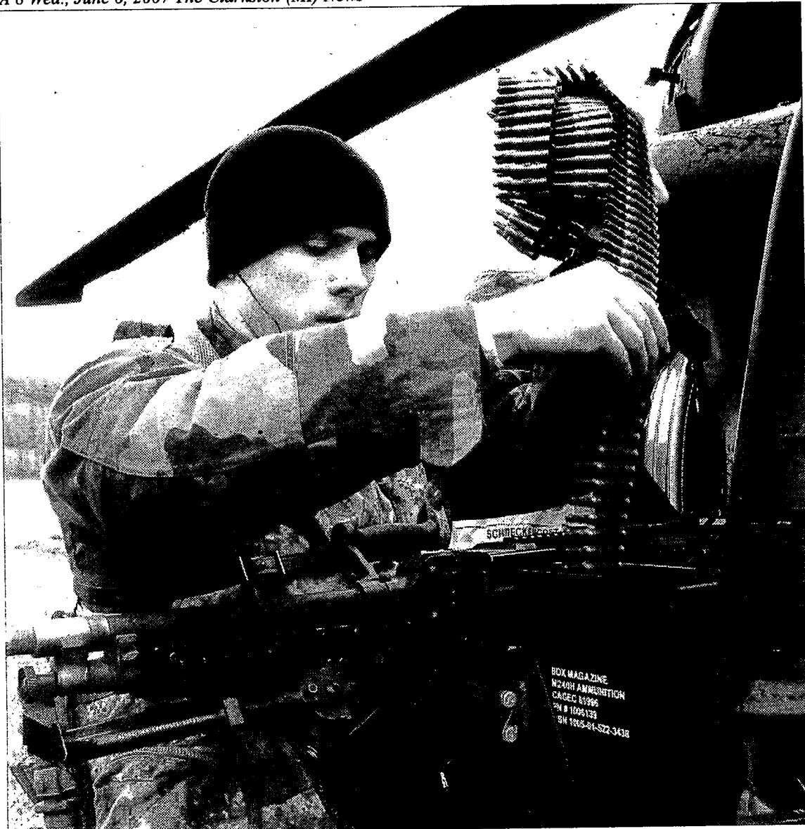
Jacob Beno feeds a belt of 7.62mm blank ammunition into his M240H machine gun for aerial gunnery training. One of his duties as flight engineer is to serve as a door gunner.
