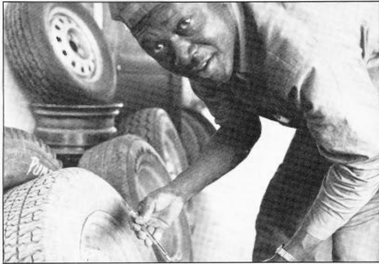
Checking with a pencil type gauge to ensure there is sufficient pressure for leak testing.
