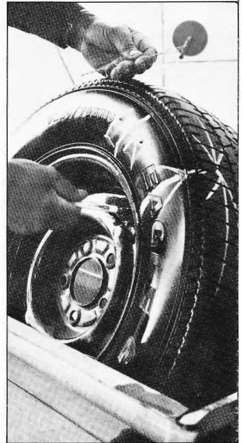
The tire must be completely removed from the rim to be repaired. To completely deflate the tire prior to demounting from the rim, Emrol removes the check valve. His left hand holds a mushroom like repair plug which will be installed from the inside and pulled through with the wire handle.
