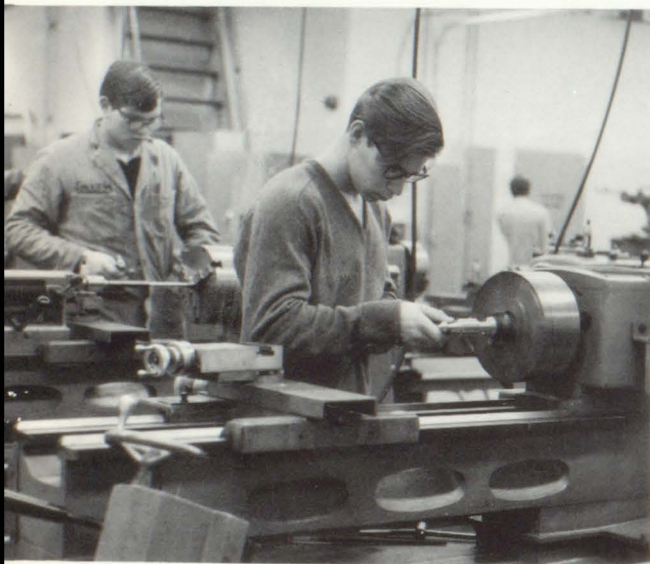
Jim Casper uses the lathe in the machine shop to hold and turn his hammer head as he shapes it, while Larry Smith holds a handle for a tap.
