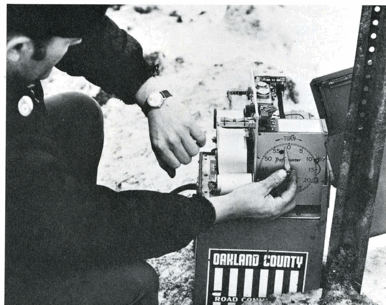
Necessary preliminary adjustments being made to a traffic counter.
