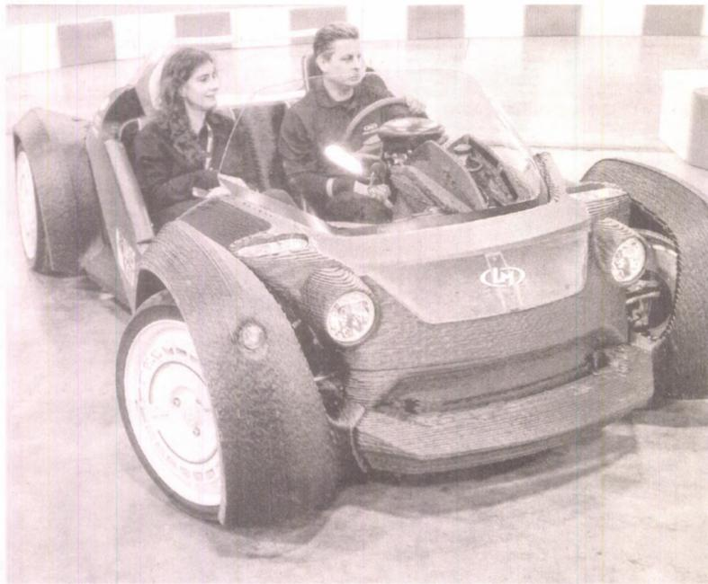
Spencer Sharp of Local Motors takes Car & Driver magazine writer Tamara Warren for a spin in the 3-D printed car.
