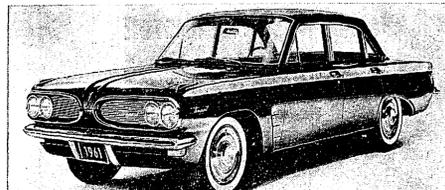
**THE TEMPEST** — Pontiac's entry in the smaller car field. It's built on a 112-inch wheelbase and features a 4-cylinder, front-mounted engine, rear transmission and an overall length of 189.3 inches. It'll be on display soon in this area at Berry Pontiac in Plymouth.
